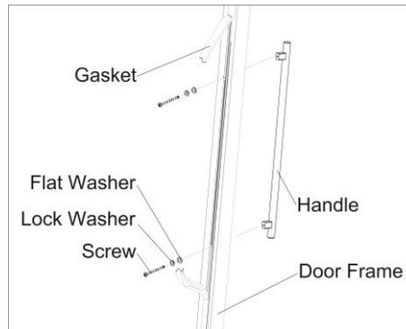
1. Remove the door gasket on the side you wish to install the handle. You can see two designated holes for handle installation.
